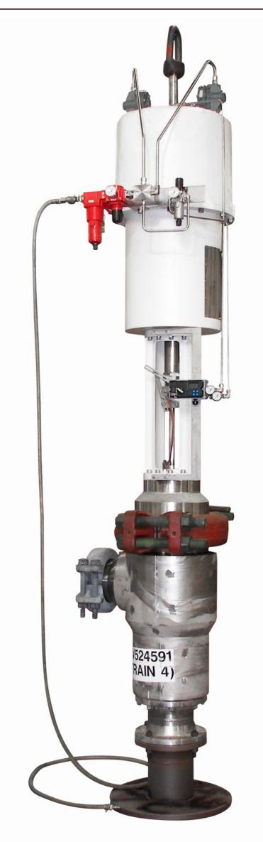
Used for both positive throttling and on/off applications on automatic control valves, Series C actuators comprise a single-spring power unit that gives distributed loadings for smooth operation. The piston is fitted with seals and operates in a 'honed' steel cylinder, delivering smooth travel and minimising hysteresis and wear.
