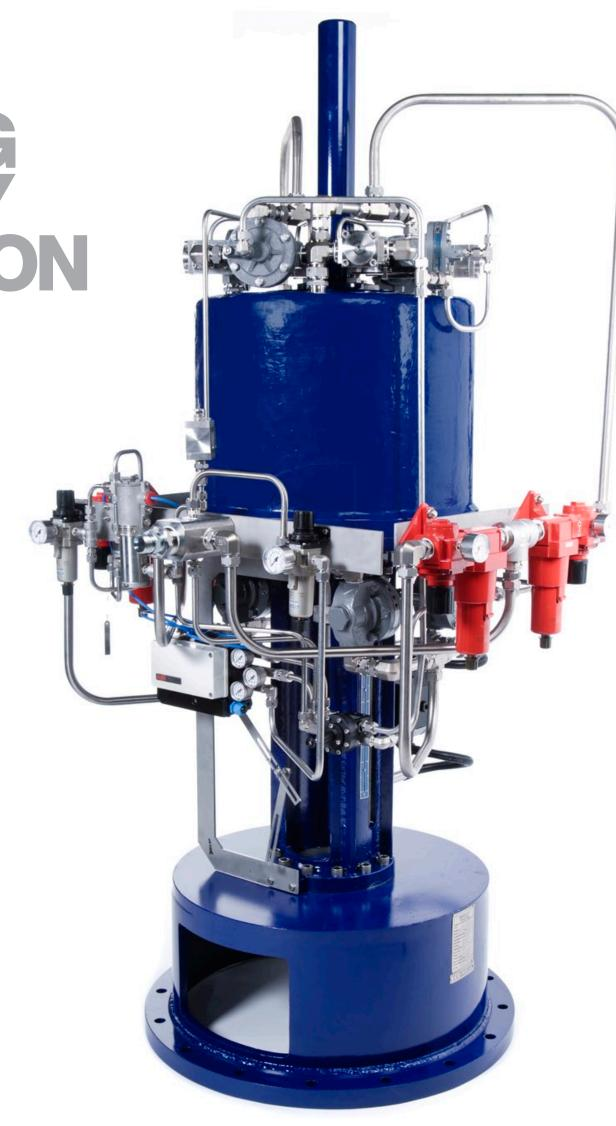
Series D actuators are created by removing the spring return feature from a Series C actuator and inserting a seal plate. This provides a double-acting piston. Extra power may be obtained for the air fail action by releasing a stored volume of air contained in a separate tank.
